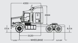
All frame height dimensions are to the top of the frame using 270mm rails.
